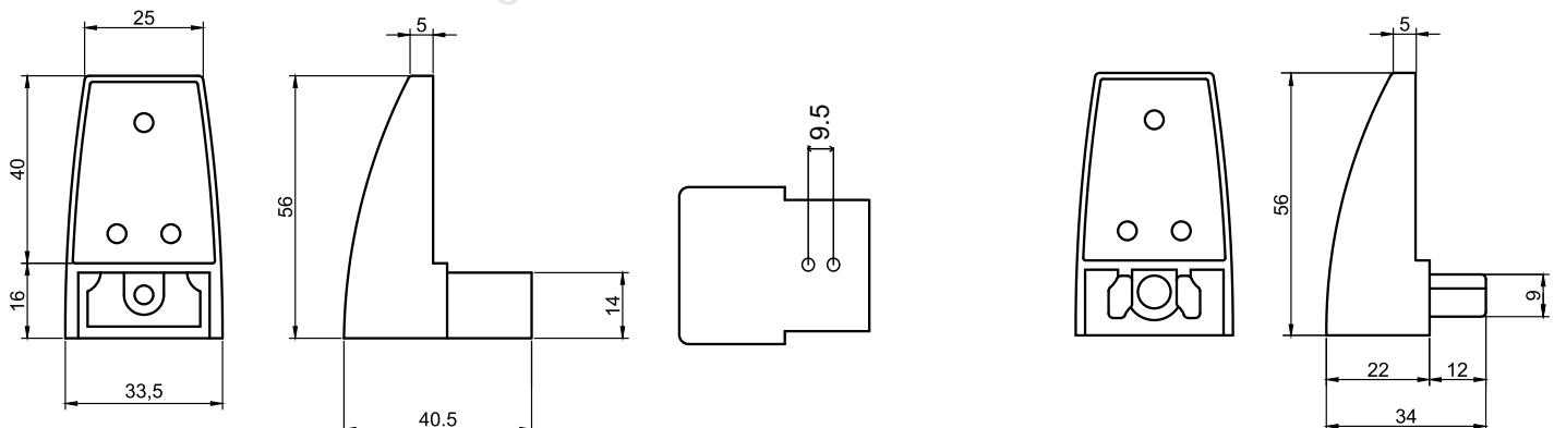
Dimensions given in this drawing are applicable prior to powder coating.
