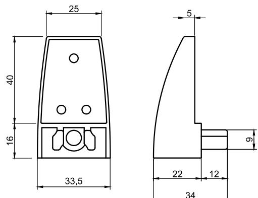
Dimensions given in this drawing are applicable prior to powder coating.
